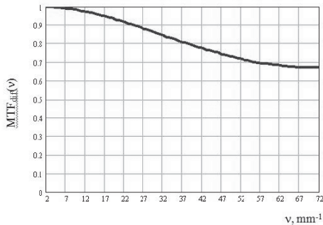
Fig. 15. Transfer inefficiency MTF for CCD
