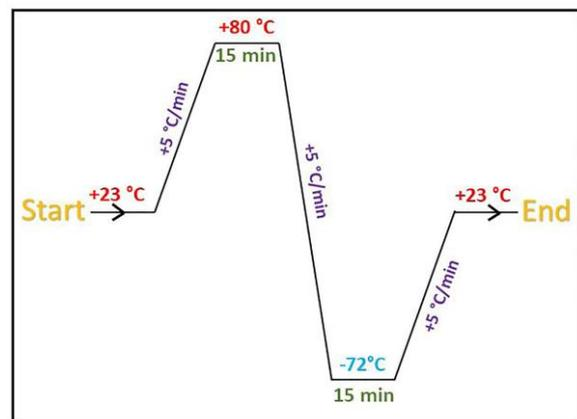
**Fig. 2.** A Schematic diagram of the temperature cycle applied to seeds.
