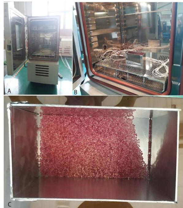
**Fig. 1.** Thermal cycling simulation of the space environment in a simulator and how to insert dry tomato seeds into the simulator. (A) A simulator for simulating the thermal cycle of the space environment. (B) A view of the interior of the thermal cycle simulator chamber illustrating how seeds are placed inside. (C) An aluminum chamber containing seeds.
