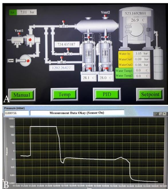
**Fig. 4.** (A) A diagram illustrating the mechanical construction of a space simulation vacuum chamber (B) and the vacuum simulation process up to 10<sup>-4</sup> mbar.
