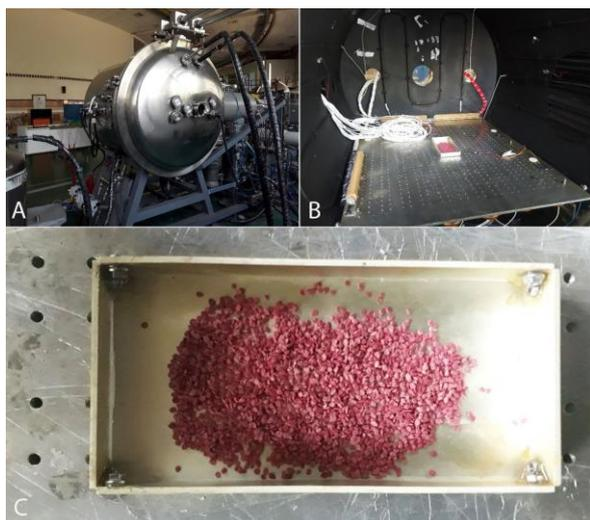
**Fig. 3.** A vacuum simulator for a space system and how to place dry tomato seeds inside the device. (A) A chamber for simulating the vacuum environment in space. (B) An interior view of the chamber used for simulating a space vacuum environment. (C) Dry tomato seeds and how place them in the chamber.
